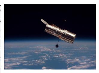
Discovery in 1990 amid huge hype and expectation. Yet after it was in position, it simply did not work, because the primary mirror was **misshapen**. It was not until 1993 that the crew of the Shuttle Endeavor arrived like roadside mechanics, opened the hatch that was installed for the purpose, and replaced the defective mirror with a good one.
